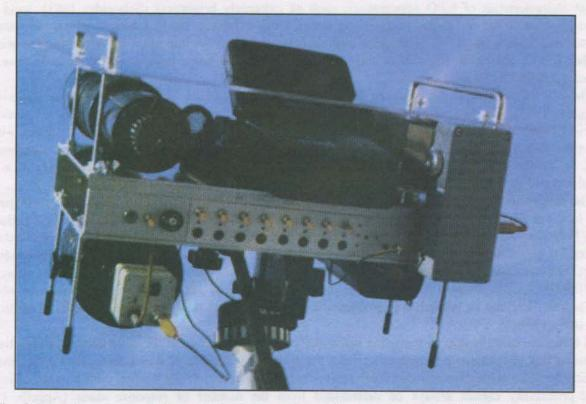
Fig. 9.4: Rear view of the optical platform for taking movies in the dark and at daylight of objects in different distances
